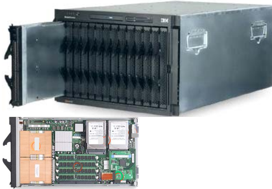
Figure 9. IBM Blade Server
