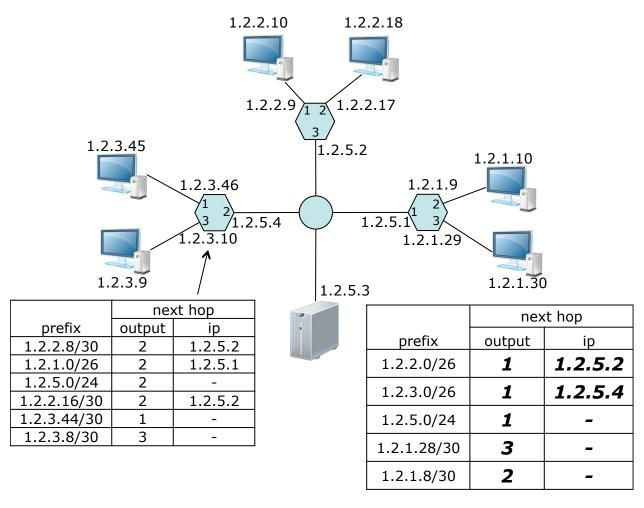
Are all the entries in the left-hand router's table necessary? If not, show how to reduce the number of entries, without changing the routing behavior.
