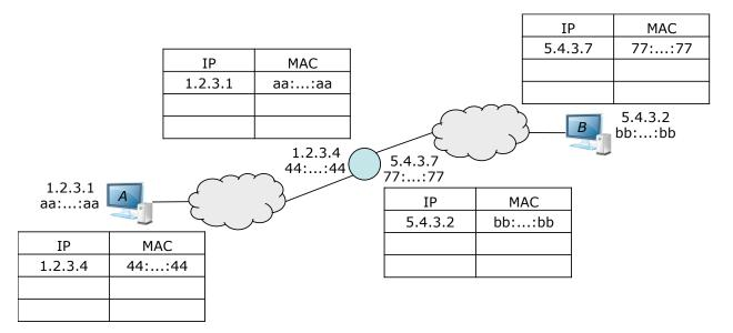
Assuming that each of the switched subnets has 100 desktop client computers and one server machine, approximately how many ARP table entries would host *A* typically have.
