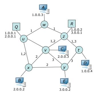
If host *B* sends a packet to host *C*, what switches and routers does the packet pass through? List them in order, repeating any switches that the packet passes through more than once.
