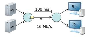
senders' congestion windows. What is the smallest value of  $cwnd_1+cwnd_2$  for which the link joining the two routers stays busy all the time?
