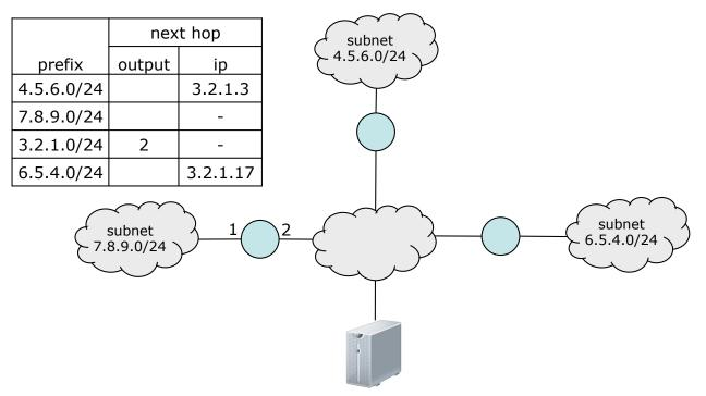
In three of the entries in the routing table, the output has been left blank. Fill in the missing values.
