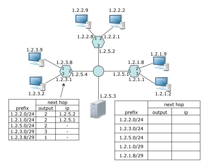
If a switch was inserted between the host with IP address 1.2.3.2 and its router, how many hosts could be *added* to that switch, without having to change the routing table entries? What IP addresses would those hosts use?
