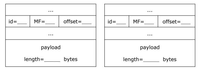
Suppose host *A* sends a 100 byte packet with the "don't fragment" flag set. Explain what happens to this packet at each of the two routers.
