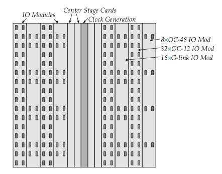
Figure 4: Physical Packaging Arrangement for ATM Switch
