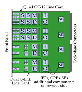
Figure 5: ATM Switch IO Module
