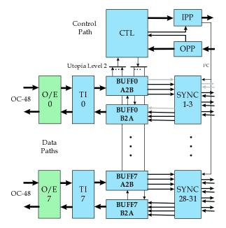
Figure 2: ATM Interface Module
