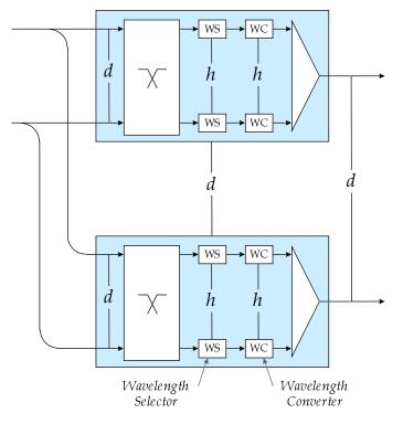
Figure 4: Optical Crossbar for Burst Switch Element
