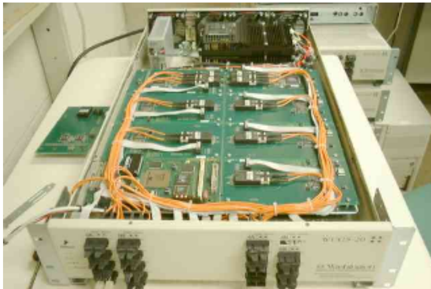
Fig. 6. Prototype environment for the DHP architecture; photograph of an FPX in a WUGS with the line card removed for visibility.
