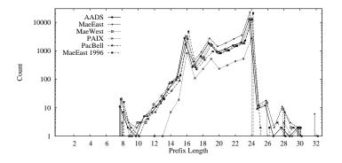
Fig. 8. Histogram of Backbone Prefix Length Distributions (log scale)
