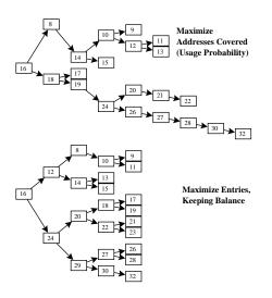
Fig. 10. Asymmetric Trees produced by two Weighting Functions
