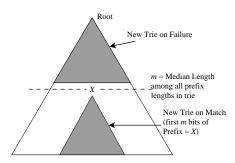
Fig. 11. Showing how mutating binary search for prefix P dynamically changes the trie on which it will do binary search of hash tables.
