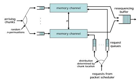
Figure 2. Multichannel buffer block diagram
