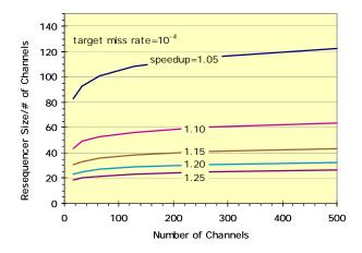
Figure 4. Scaling of resequencing buffer size
