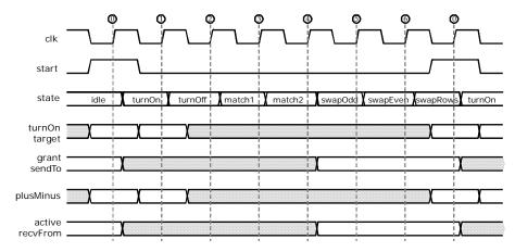
Figure 5. Timing of IO and internal operations
