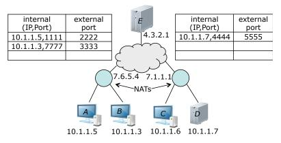
Show the values of the address and port fields in the diagram below, for a typical packet sent by host *A*.
