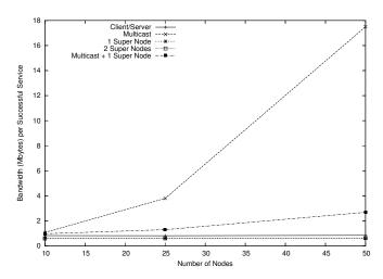
**Figure 8**. Network traffic per successful service as the star topology increased in size, with the multicast configuration providing the most expensive service per megabyte solution
