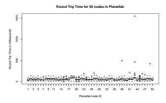
Fig. 6: Round Trip Times from each node to all 50 nodes in Planetlab.
