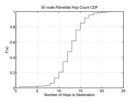
Fig. 3: CDF of the number of hops necessary for nodes to reach each other in the 50 node Planetlab experiments.
